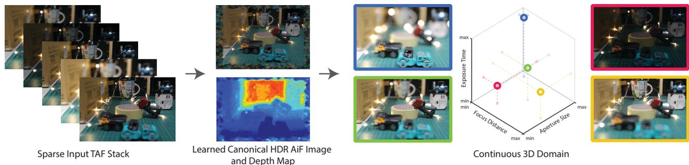
Fig. 1. Our approach is capable of accurately reconstructing a canonical all-in-focus (AiF), high-dynamic-range (HDR) radiance map alongside with depth information, using a sparse Time-Aperture-Focus (TAF) stack as input. This gives full post-processing control over focus, aperture, and exposure conditions.
